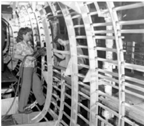
Women Assembling an Airframe, One with a Rivet Gun, Courtesy of San Diego Air and Space Museum.
